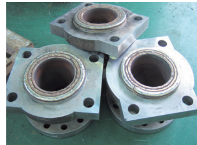
Weld built up (ASME Sec IX)
