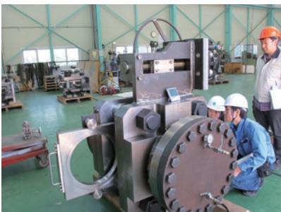
Pressure Test (API 598)
