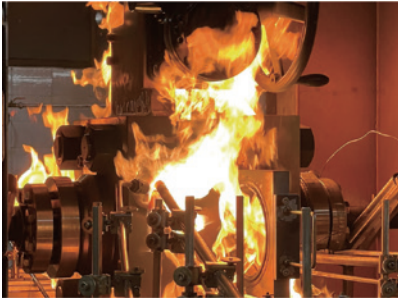
Fire Safety Test (API607)
