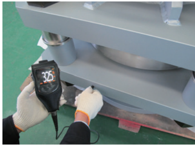
Dry Film Thickness Inspection (ISO 19840)
