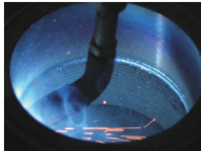
Weld Built up
